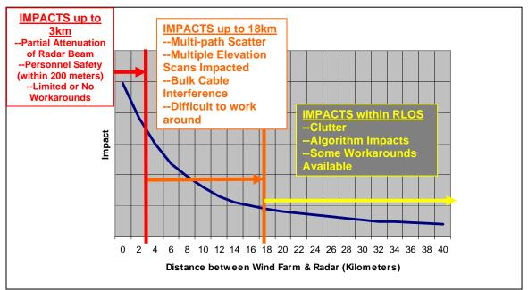
Fig 2. Notional impact of wind farms on NEXRAD radars relative to the separation distance.
