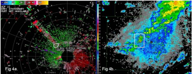
**Fig 4a.** This Velocity image (0.5 degree scan) from the Great Falls, MT WSR-88D (KTFX) on February 9, 2006 at 1859 GMT shows how only a few turbines very close to the radar can cause a relatively large impact. The 6 turbines are approximately 6 km from the WSR-88D and in the RLOS. The velocity data is contaminated in azimuth for 9
